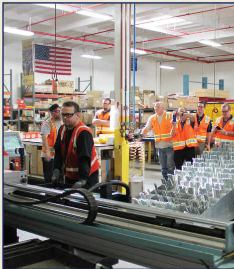
Brandon Crick is shown here operating the Scotchman automated all thread cutter in Murray's hanger department. Once the all thread is cut, it is then assembled onto hangers and/or racks which are then labeled and packaged to meet the specific project requirements. Brent Mitte (to the left of Brandon) explains how the machine operates and how it has increased Murray's production
